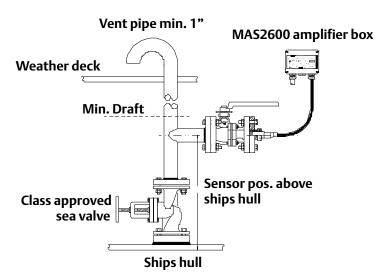
Transducer measuring range > max. draft minus sensor position.
